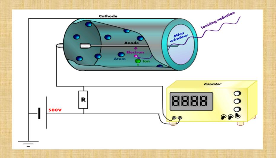
Geiger tube consists of a wire anode surrounding by a mental cathode, the space between them being filled with a mixture of gases (often argon or neon with a little bromine or chlorine) at low pressure. There is usually a small glass bead on end of the wire anode to prevent discharge from a point.
